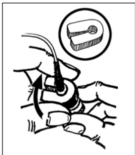
Tool for tightening MicroDot connector firmly to Miniature Power Supply.
